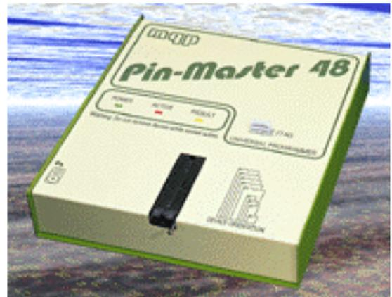
The PM48 programmer is controlled by an internal microprocessor. On power up the software is downloaded from the PC to the programmer. Software upgrades only involve installing the latest version onto the PC. The design features re-configurable logic, and allows: any voltage on any pin, power supplies on any pin, programmable slew rates, and voltage measurement of any pin.
