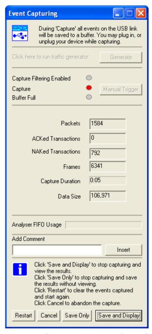
When saving the capture file, you can click 'Save Only', and the file will be saved without the need to perform the normal display parsing. On very large files this can result in a considerable time saving.
